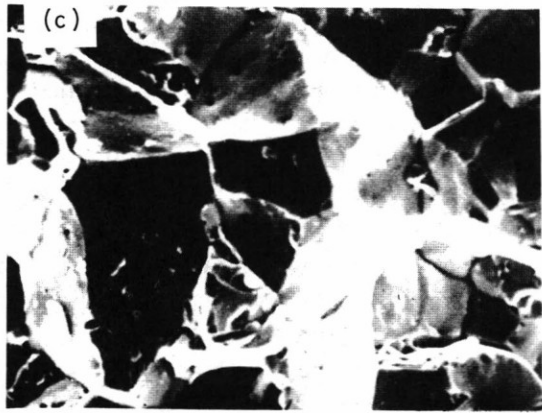
Fig. 5: a) A sample of failed springs (x0.5). b) A characteristic fracture of a coil. Areas A, B are intergranular. Cadmium penetrations were detected along the arrowed edge (x15). c) SEM micrograph of the intergranular structure of area A (x4000).
