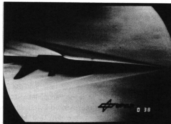
FIG. 12: SÄNGER test model in the DFVLR shock tunnel Göttingen at Ma = 6.8
