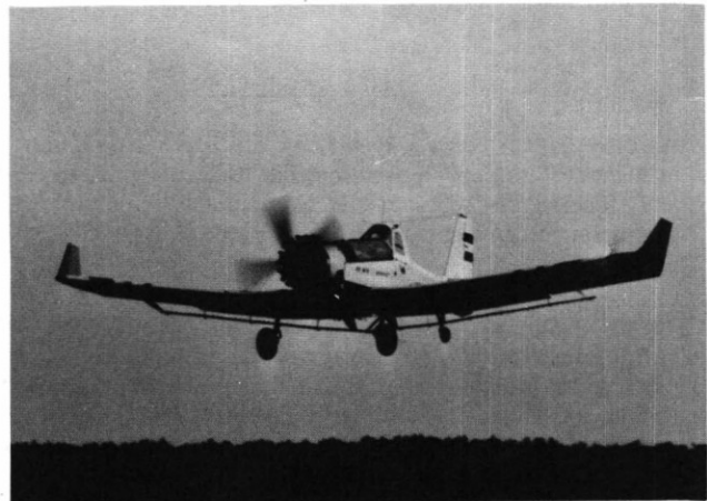
Figure 5. PZL M-18 fitted with winglets
