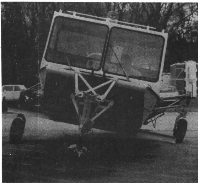
Figure 2. Airboat Test Frame for Tilt Steering Research
