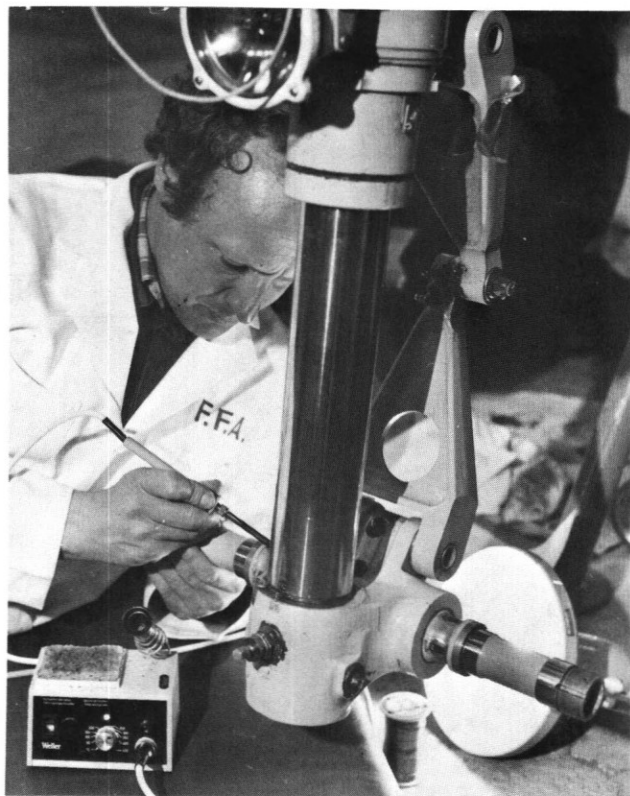
FIGURE 3 SF-340 nose gear shock strut during strain gauge application
