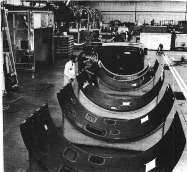
Figure 1. CFC fan cowl doors for RB211 engine
