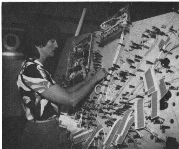
FIGURE 8. Conventional Wire Bundle Routing
