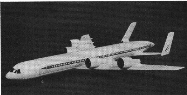
Figure 19. Flatbed with Passenger Module
