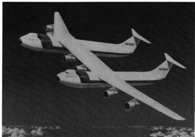
Figure 7. Multibody Cargo Transport Concept
