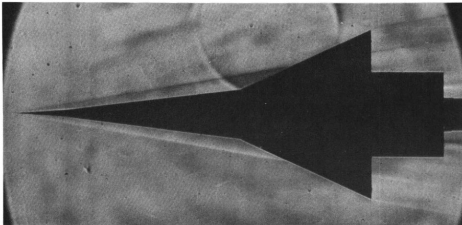
Fig. 11 Schlieren photograph of the flow around the HST model without fences ( \alpha = 2^\circ ).
