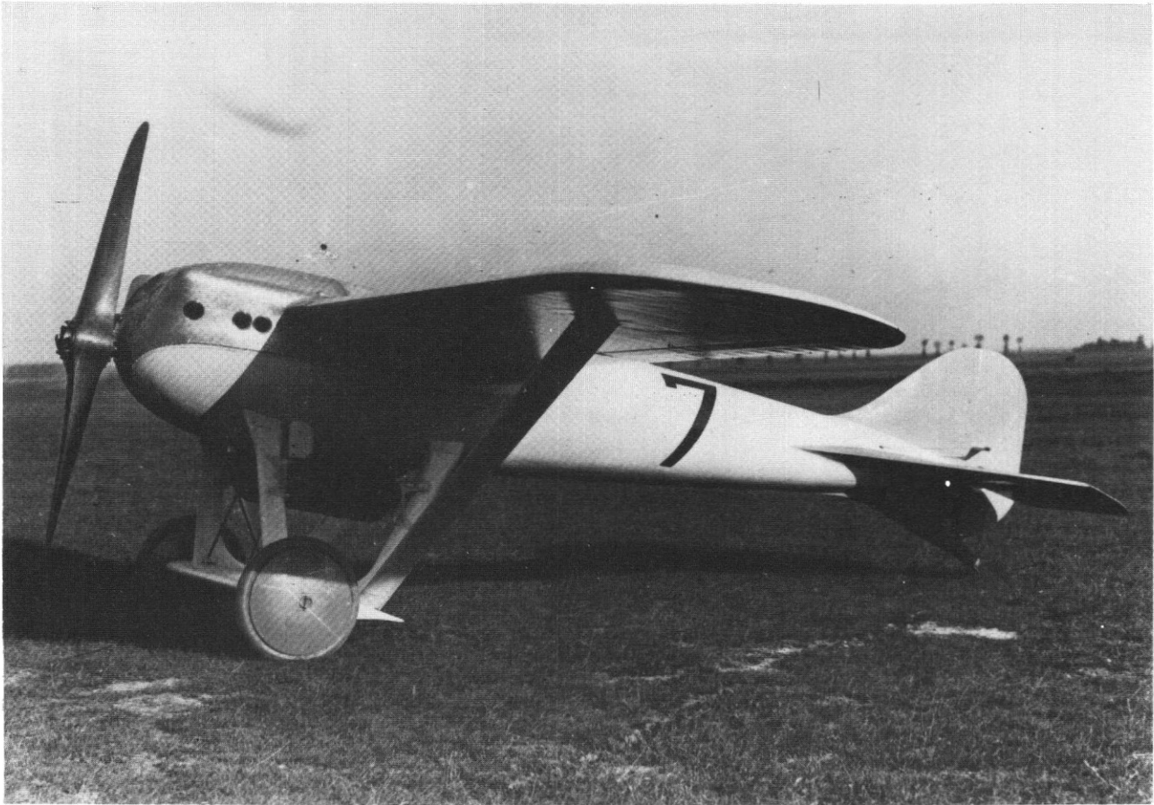
11 — Nieuport sesquiplane fitted with Lamblin radiators. 1921.
