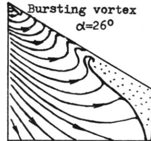
Flow patterns on upper surface ( \alpha=18^\circ \alpha=26^\circ )
