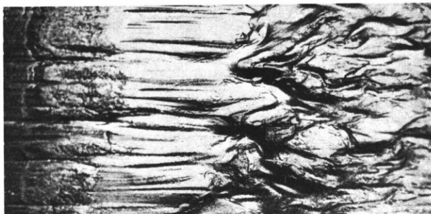
Photo. 4. A post-test wax model Re/m = 7.5 \times 10^7
