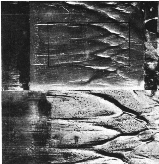
Photo. 2. A post-test wax model Re/m = 4.7 \times 10^7
