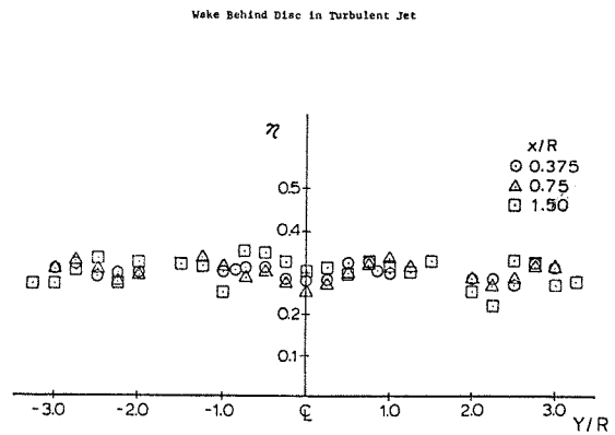
Figure 7. Turbulent Intensity Profile Summary, 2 inch Diameter Disc
