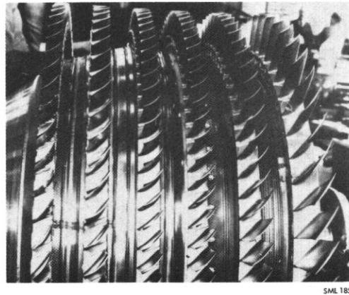
Fig. 15 HP Compressor End Bend Rotor
