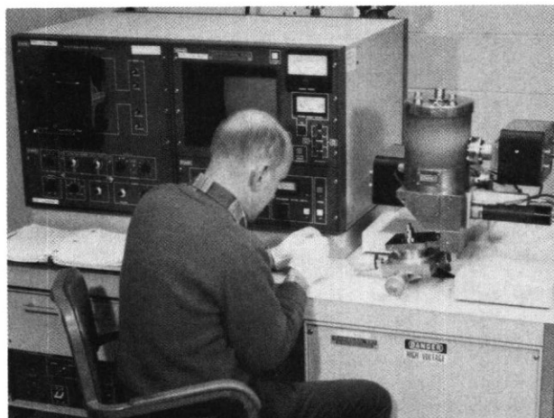
FIGURE 2. Mounting specimen in scanning electron microscope for detailed examination.
