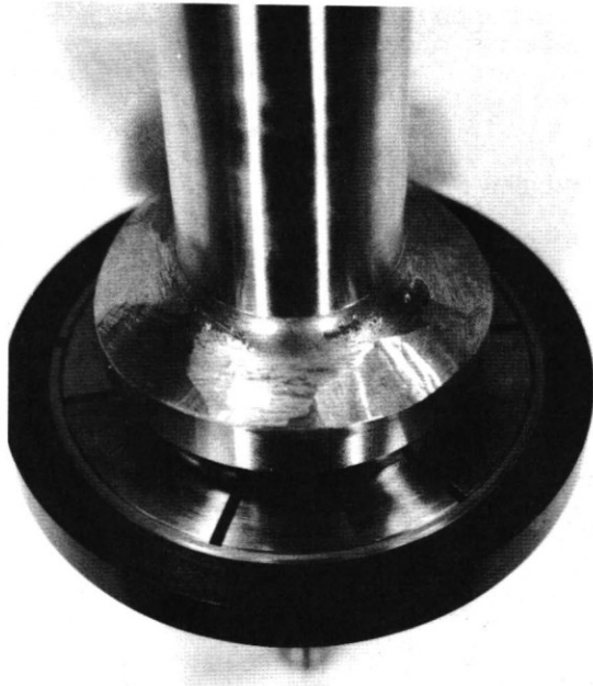
Fig. 12: Cold spin test device for ring qualification
