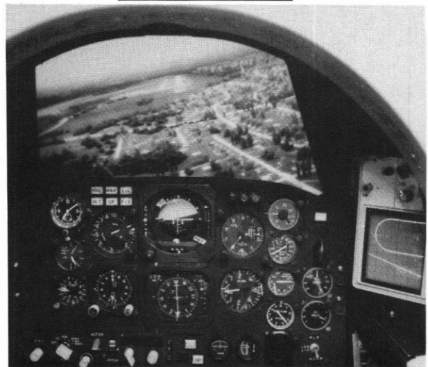
Figure 6. Picture of the instrument panel, including the pictorial display and simulated outside view
