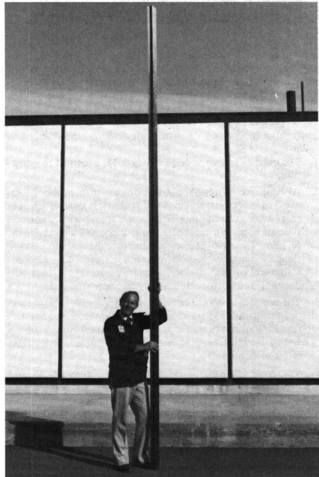
Fig. 27 Full-scale, 18-foot, composite hat/skin component.
