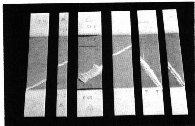
FIGURE 24 - TYPICAL FAILURES (MODE 2)
