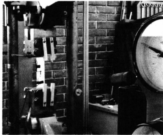
FIGURE 18 - SWINGING GRIPS FOR FLAT SPECIMENS
