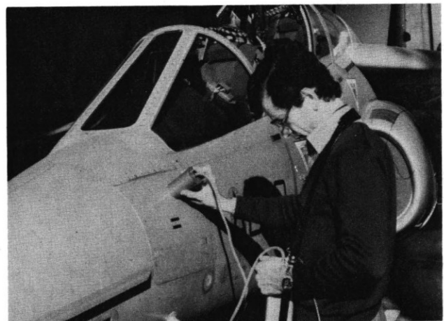
Fig. 3 - Using the CORAS for verification of bonding.
