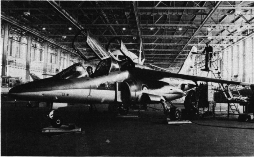
Fig. 6 - Simulating static charging on an aircraft
