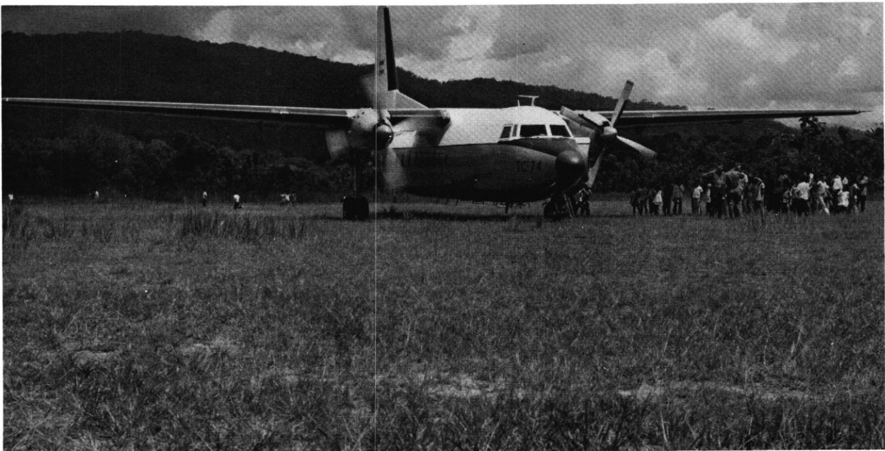
Fig. 2 Fokker F27 "Friendship", of which the operational life may be extended to 90.000 flights, operating from a typical poorly paved airstrip.
