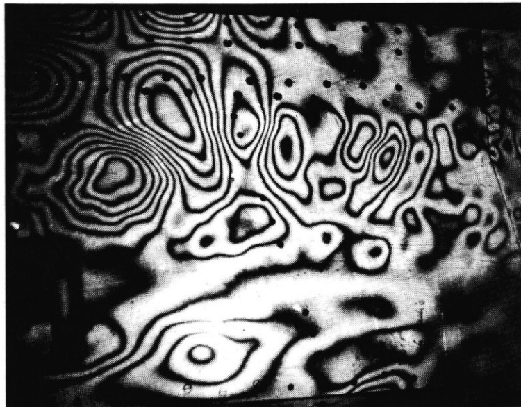
Figure 14. Holographic visualization of the field of deformations in a wing element. \tau = 1 ms. \Delta t = 3.3 \mu s. Without kerosene
