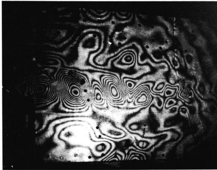
Figure 13. Holographic visualization of the field of deformations in a wing element. \tau = 1 ms. \Delta t = 3.3 \mu s. With kerosene filling the interspaces
