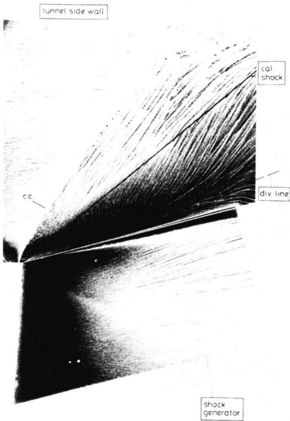
Fig. 7 Oil-Flow Picture at \delta_s = 15^\circ
