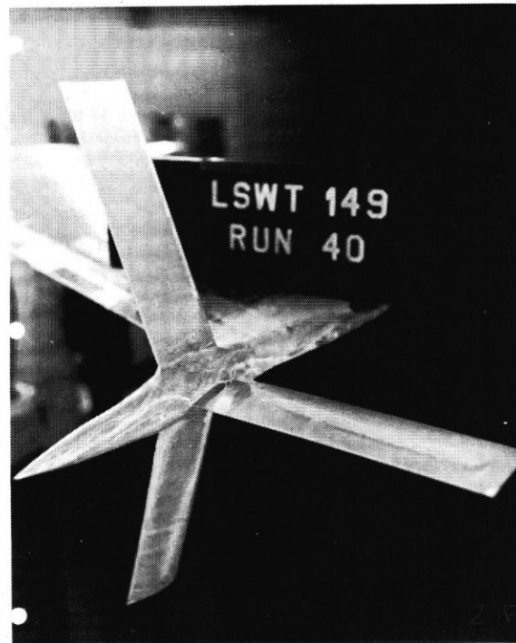
Figure 12. The Three-Vane Vortex Diffuser, Showing Surface Flow
