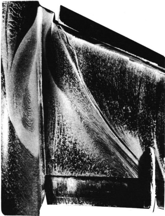
FIG. 29 WING ROOT FLOW AT STALL - 90% SPAN SLAT.
