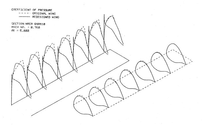
Fig. 10 Shock-free redesign of a rectangular wing with NACA 64A410 section.
