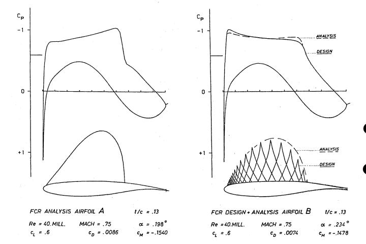
Fig. 5 Shock-free redesign with constant thickness for prescribed Mach number and lift coefficient, including viscous effects.
