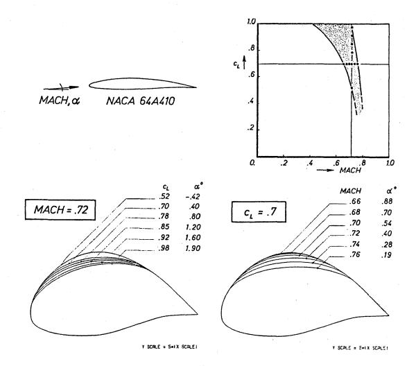
Fig. 3 Inviscid design example: Shock-free flow modifications of NACA 64A410 airfoil.
