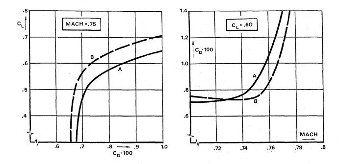
Fig. 6 Comparison of original and redesigned airfoil: lift, drag, Mach number.
