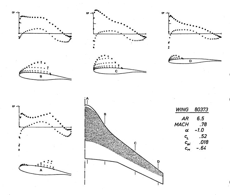
Fig. 11 Shock-free design of a swept wing.
