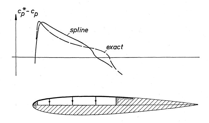
Fig. 8 Shock-free modification of NACA 0012 airfoil, elastic section approximation.
