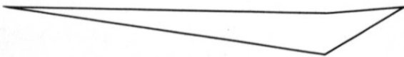
Fig. 16 Optimum double-wedge profile of minimum heat transfer of given lift coefficient and cross sectional area
