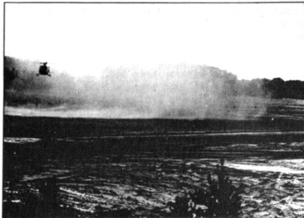
FIG. 8 DUST CLOUD PRODUCED BY A SCOUT HELICOPTER AT 6M HEIGHT
