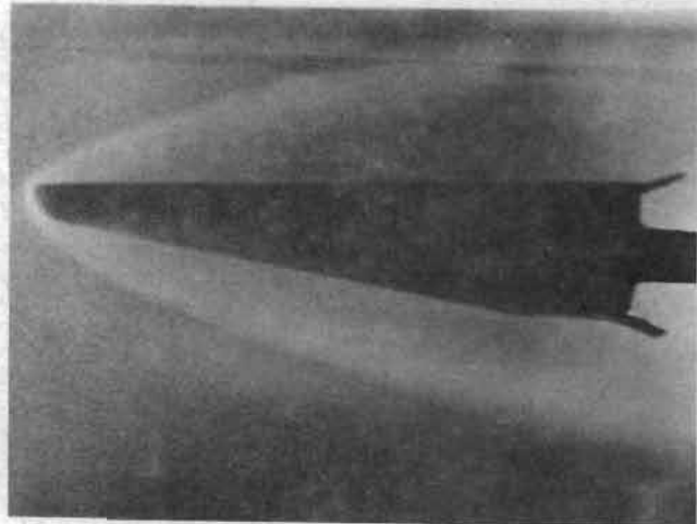
Figure 8. Shock wave pattern around an Integral Body visualized by glow discharge.
