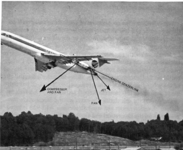
FIGURE 1. NOISE SOURCES OF A TURBOFAN ENGINE
