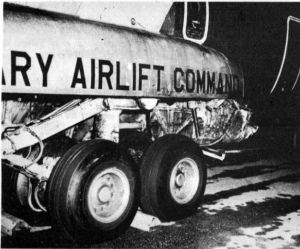
Fig. 14 - C-141 Main Landing Gear Fairing Damage
