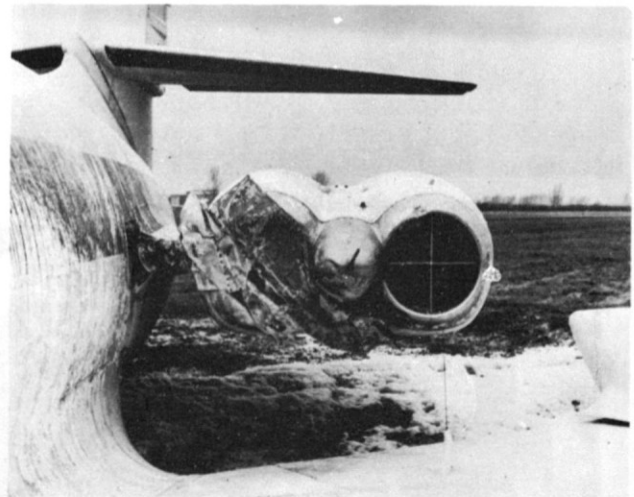
Fig. 17 - Result of In-Flight Collision Involving C-140
