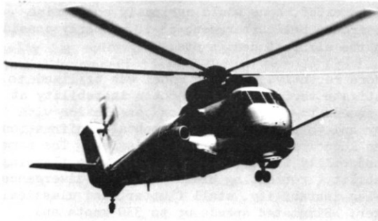
FIGURE 13. NH-3A RESEARCH HELICOPTER WITH JET THRUST AUGMENTATION
